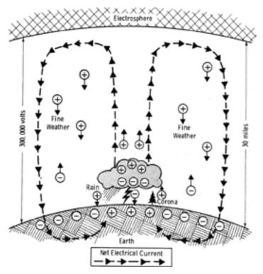
Figure 18.1: Thunderstorms act as batteries to keep the earth charged negatively and the atmosphere charged positively. Atmospheric electrical currents flow downward in fine weather and upward in thunderstorms. Thunderstorms deliver charge to the earth by lightning, rain, and corona discharges.
