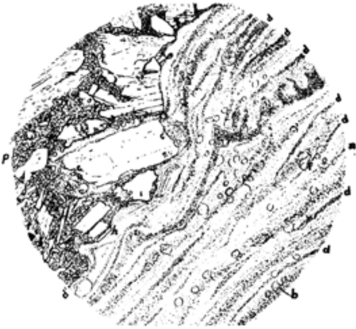
Figure 3: Rock-Fulgurite, Wyoming. X 50. Cross-section of contact.
